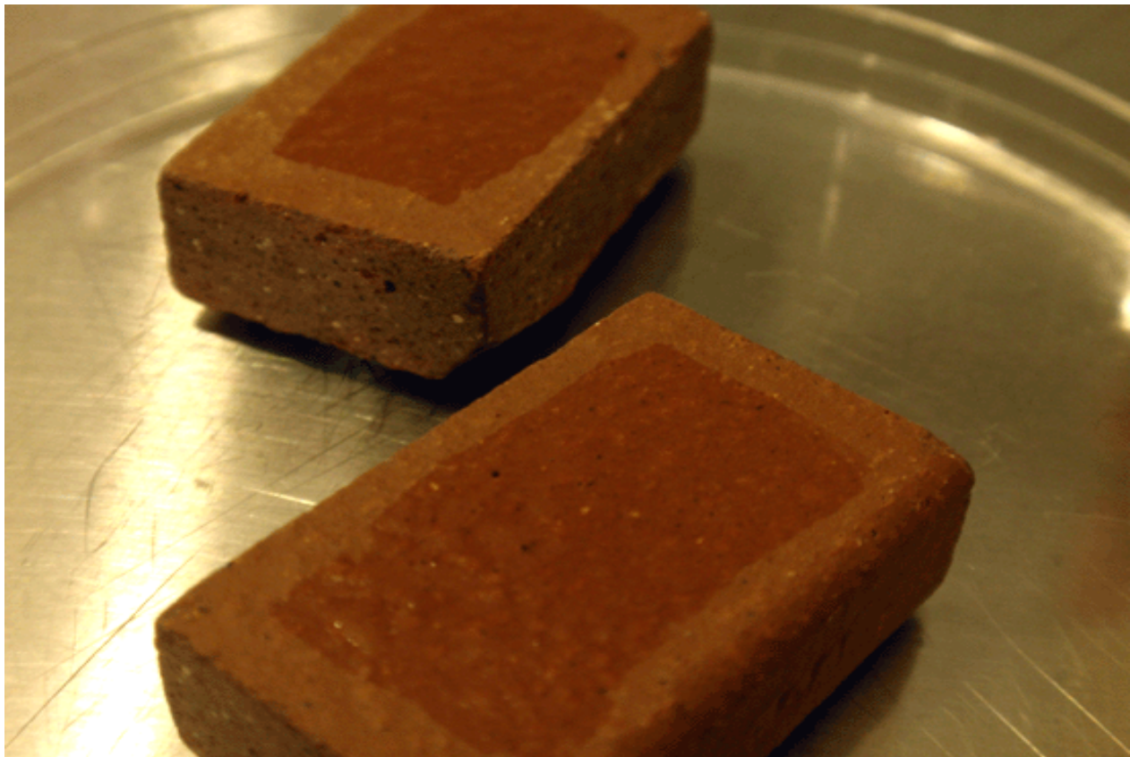
Test carriers inoculated with the test organism prior to treatment with cleaning instrument.
